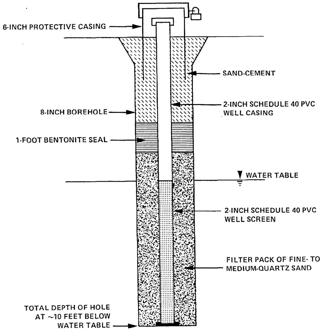
FIGURE A-1. Recommended Monitoring-Well Construction
