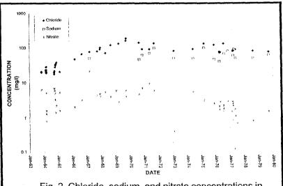
Fig. 2. Chloride, sodium, and nitrate concentrations in well G from 1963 to 1979.
