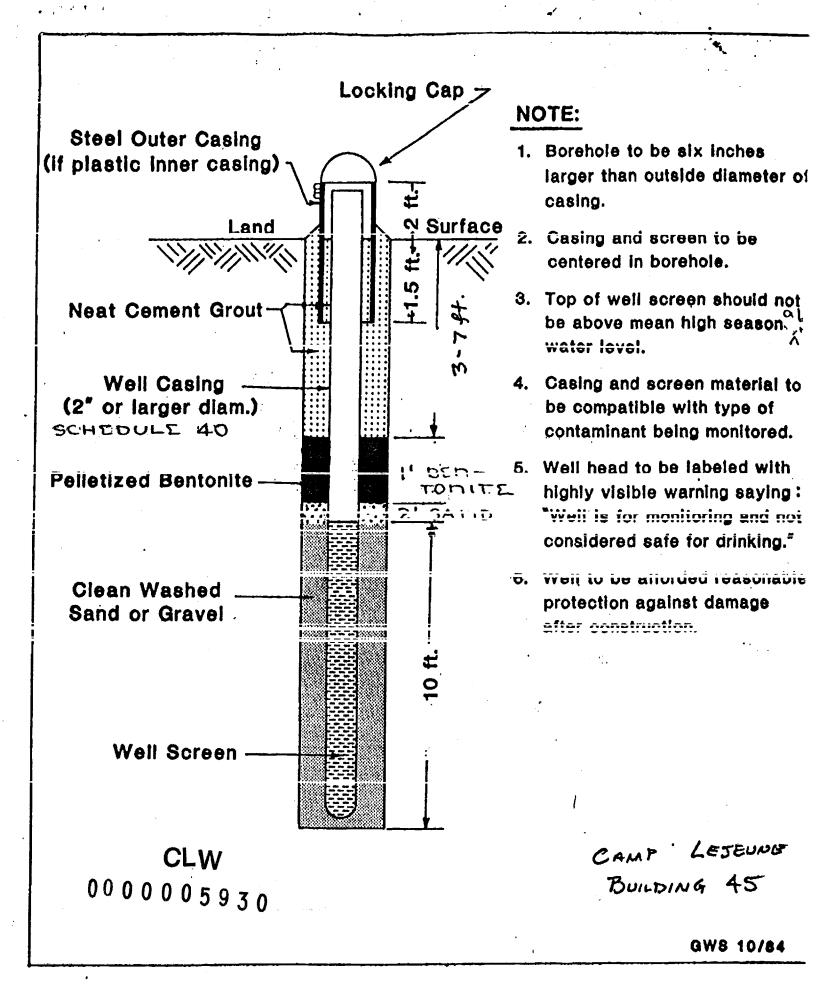
Recommended Construction Details For A Contaminant Monitor Well to An Unconfined Unconsolidated Aquifer
