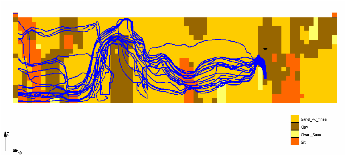
Figure 6.9 Side view of flow lines and water table.
