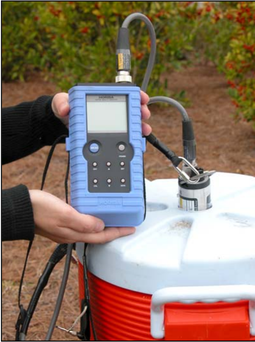
Figure 4. Photograph showing HORIBA W-23XD water-quality control unit and cable attached to dual probe ion detector housed in a protective plastic 5-gal water jug
