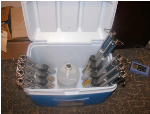
Figure 6. Photograph showing use of a water bath for calibrating multiple loggers.
